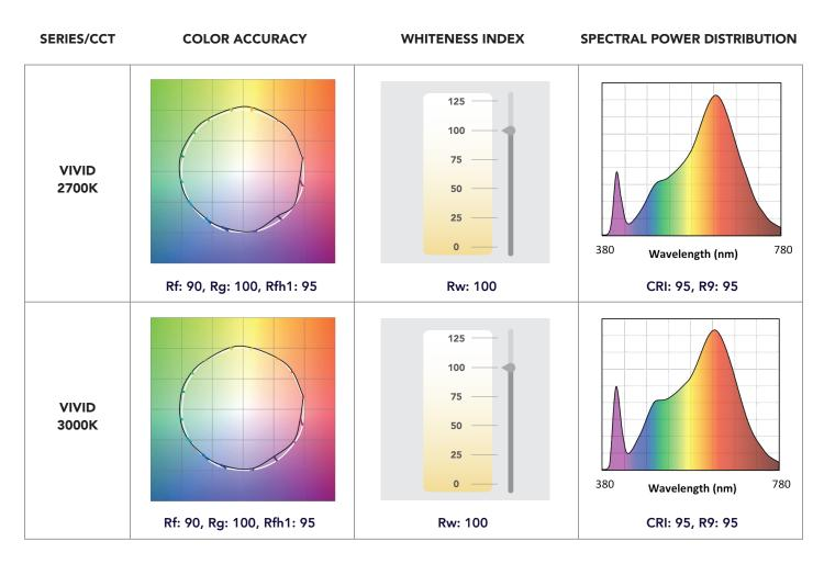
Rf: TM-30 metric measuring color fidelity (whether colors are similar to those under natural light). Rf is a more accurate version of the CRI Ra. Rf is 100 for natural light. Rg: TM-30 metric measuring color gamut (whether colors are more saturated than under natural light). Rg is 100 for natural light.
