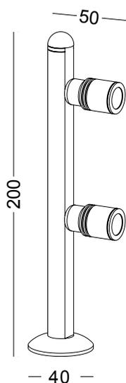
installation IP20 cut-off dia 10mm hole for installation / maximum 25mm thickness board
